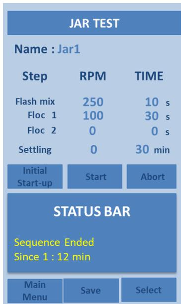
15. The Status Bar will then show "Sequence ended". The RPM and the timer indicate zero.
