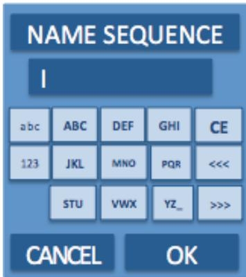
This display is used to enter letters, numbers and symbols as needed when programming the instrument. Unavailable options are disabled (greyed out). The icons on the right and left of the screen are described in Table 5.1.
