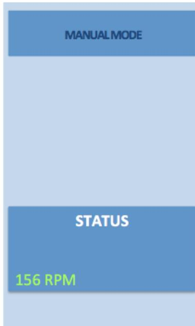
**Manual mode** allows manual operation of the mixing, regardless of the programmed sequence (flash mix, flocculation and settling). The user controls the speed and time desired for each step of the test.
